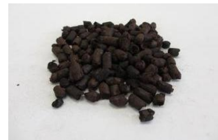
Semi-carbonized pellets made of bark of Cryptomeria
