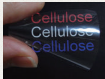
Transparent sheet made from cellulose nanofiber
