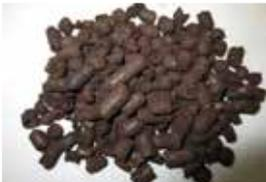
New woody biomass solid fuel made with torrefaction technology
