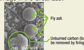
Fly ash from Nippon Paper Industries' Ishinomaki Mill. Electron microscope image of fly ash (prior to firing)
