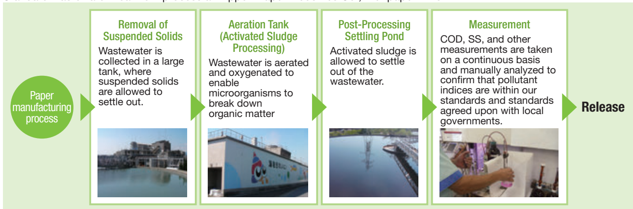
Standard wastewater treatment process at Nippon Paper Industries Co., Ltd. paper mills
