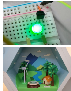
(Top) An LED lit by a CNF electricity storage body (Bottom) Display at Expo 2025 Osaka, Kansai, Japan
