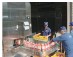
Using a filling machine to check carton quality at the Liquid Packaging Center
