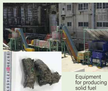
Solid fuel produced from wastepaper residues
