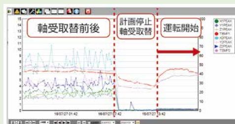
An example of monitoring using the e-wireless patrol system
