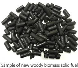
Sample of new woody biomass solid fuel
