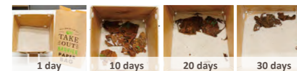
Biodegradability Test Results for SHIELDPLUS® Square-Bottom Bags
