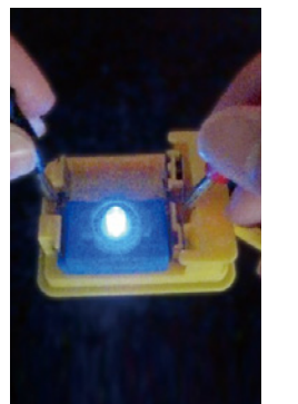
LED lighting that relies on a CNF-based electricity storage body
