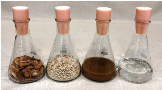
Bioethanol production process (from left to right: wood chips, pulp, saccharification and fermentation culture medium, bioethanol)
